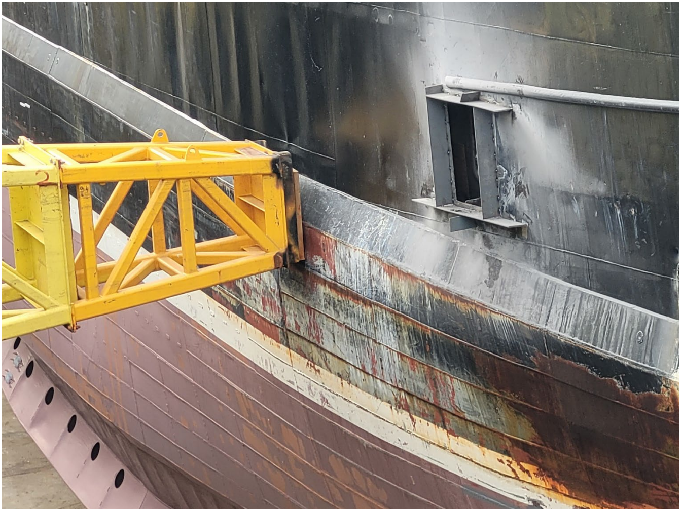
Figure 15: Photo of Sidewall Support Arm Showing Sidewall Engagement
